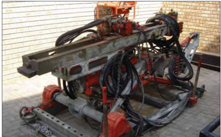
Photograph taken of the drilling machine after 4 months operational conditions, illustrating the comparisons between uncoated bolts, painted surfaces and the hot dip galvanized machine components.
