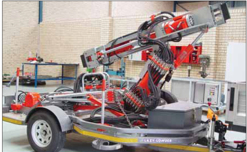
Mobility of the equipment, to the mine site as well as underground, was an important feature and therefore incorporated into the design.
